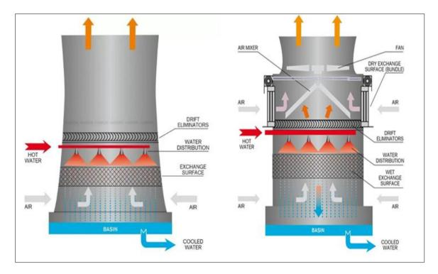
Figure 8 (a): Natural draft cooling tower (b): Induced draft cooling tower
