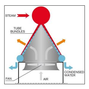
Figure 9: Dry Cooling Tower (Bushart, 2014)
